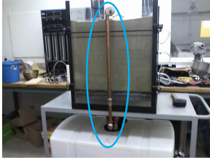
FIGURE 53. Long pipe connected to wall fitting to bring overflow to water reservoir.
