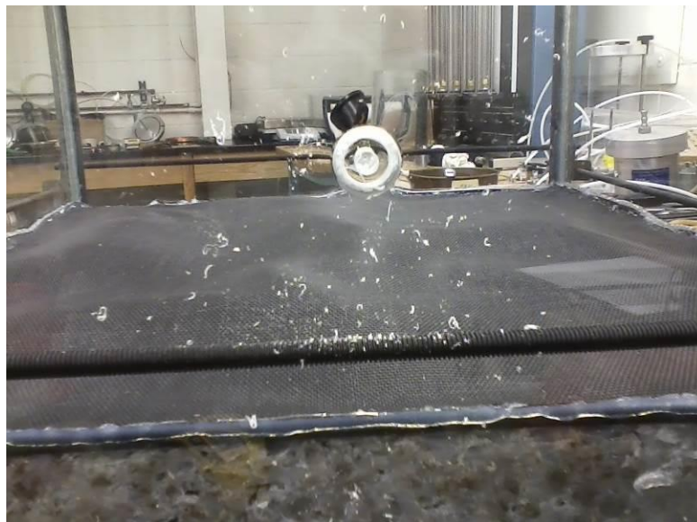
FIGURE 55. Holes being drilled for piezometers.
