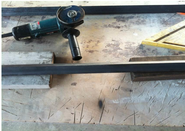
FIGURE 30. Angle beams to be cut for manufacturing of support braces.
