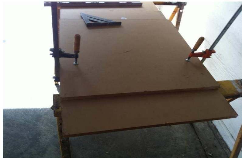
FIGURE 10. Table clamps used to secure acrylic boards during cutting.
