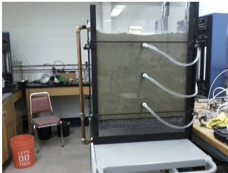
FIGURE 57. Side view of wall with piezometers.
