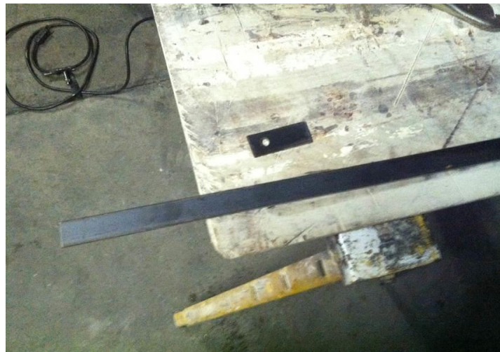
FIGURE 31. Flat steel beam used to make tabs for retaining structure.
