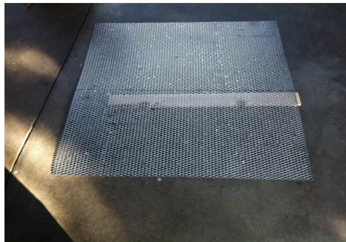
FIGURE 38. Galvanized steel mesh to resist corrosion from water.
