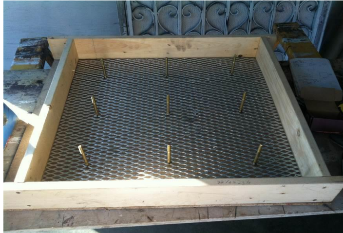
FIGURE 39. Mold with steel mesh and bolts install in the lower portion.
