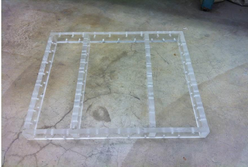
FIGURE 44. Base to sit the porous stone inside the tank.
