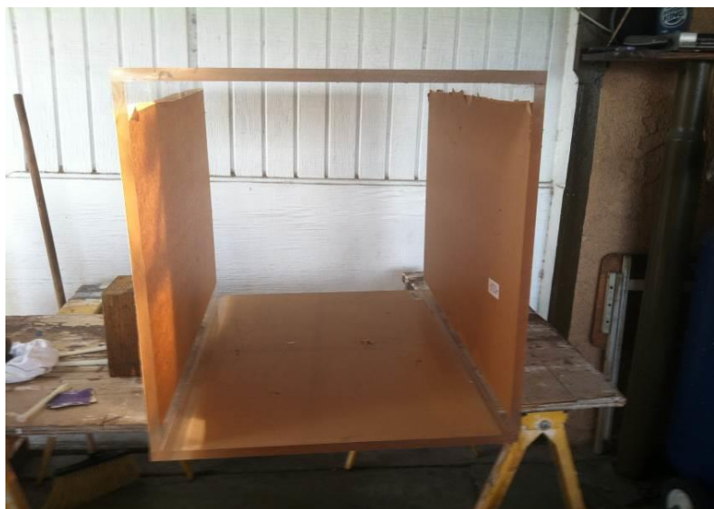
FIGURE 17. Gluing of third wall.
