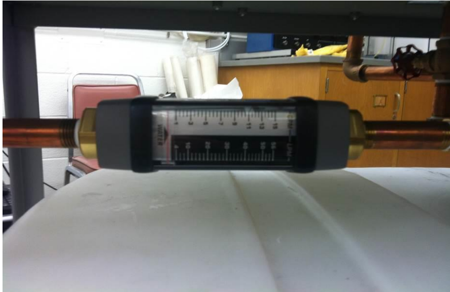
FIGURE 48. Flowmeter for measuring water flow rate into the liquefaction tank.
