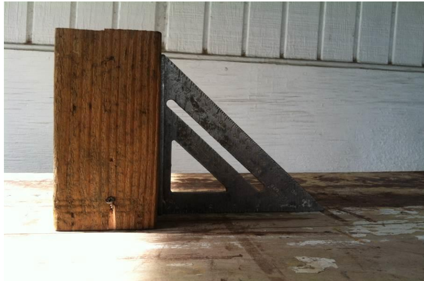
FIGURE 13. Table jig to create a squared inclined surface.
