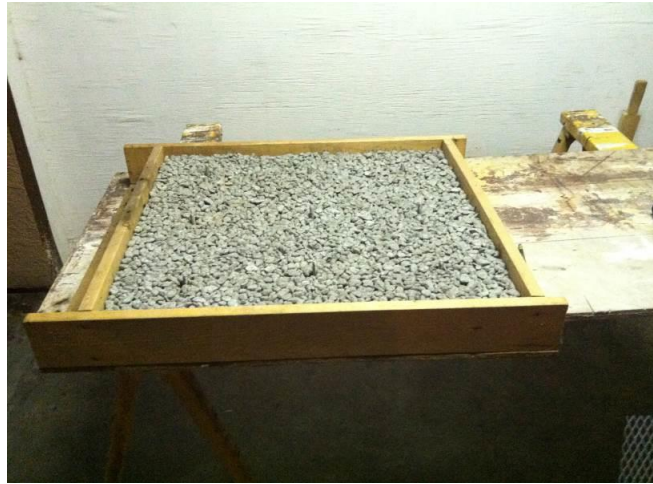
FIGURE 41. Mixture casted into mold.
