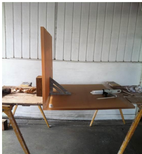
FIGURE 15. First wall glued together on the inclined work table.
