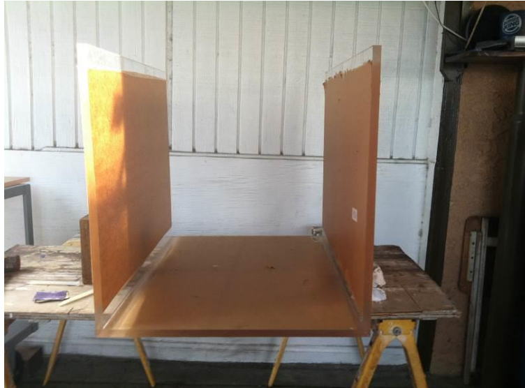
FIGURE 16. Gluing of second wall.
