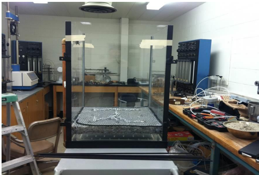
FIGURE 34. Braces fitted onto the tank prior to installation of tie rods.
