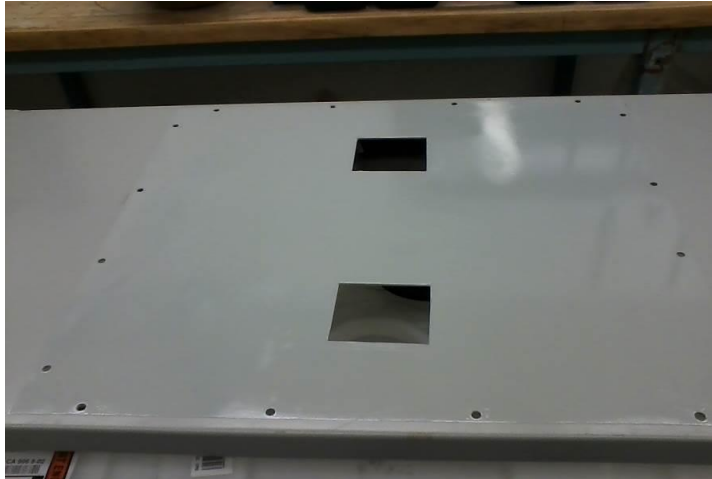
FIGURE 22. Square holes for the installation of a drain and water pipe.
