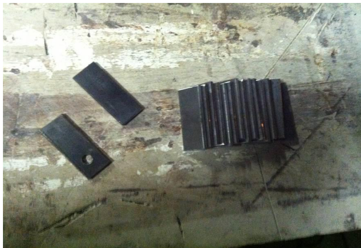
FIGURE 32. 16 flat steel tabs for the installation of tie rods.
