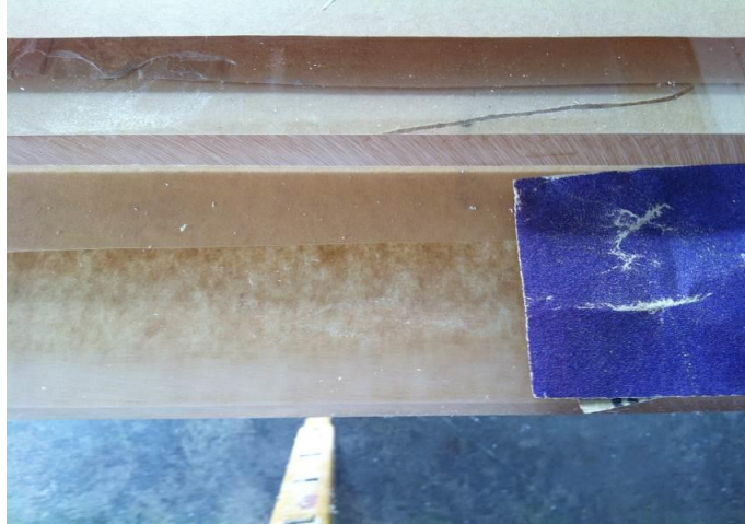
FIGURE 14. Mating surface sanded for proper gluing contact.
