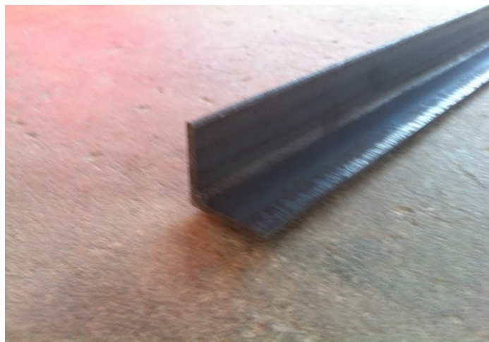
FIGURE 23. Angle steel for tank base prior to cutting.
