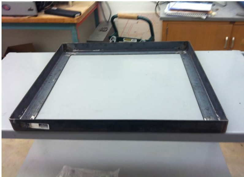
FIGURE 25. Welded base on the cart prior to hole drilling.
